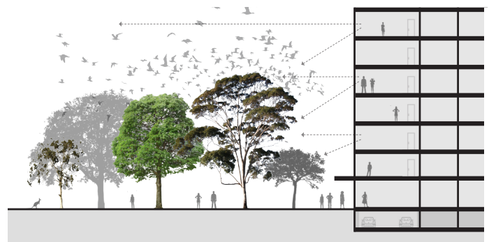
Figure B2.1. Development cross-section demonstrating how residents can maintain connection to the natural world in mid-rise development. This connection is broken above 5 storeys. Image: Simon van Wijnen.
